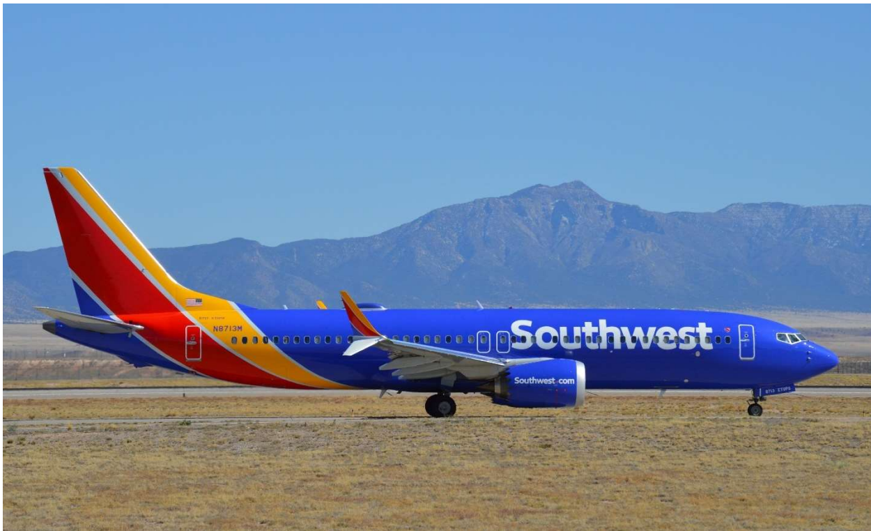
Southwest Boeing 737-8 Max at Albuquerque. The aircraft is very similar to the 737-800 but is equipped with the latest technology “LEAP” engines manufactured by CFM International.
