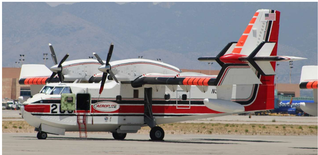
AeroFlite Bombardier CL-415 is the type of aircraft used to scoop water from Heron Lake in June, 2022.
